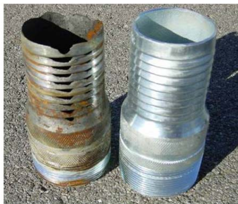
Figure 1. (Left) a corroded pump fitting that required replacement after one day of operation using sodium persulfate. (Right) a new fitting for sake of comparison.
